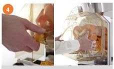
Remove the front cover screws & take off the Front Cover. Not
