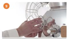
Take off the fruit supply tunnel by opening the fixation lever.
