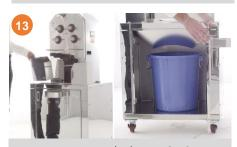
Remove the peel chutes & if available the bucket below. (clean the peel disposal area)
