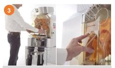
Remove the splash protector & the side chutes by pressing the fixation clip.
