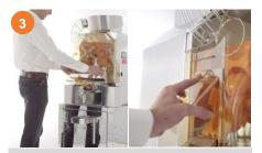
Remove the splash protector & the side chutes by pressing the fixation clip.
