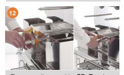
Remove, disassemble SB-Tap by unscrewing from machine. Remove fruit sieve holder (open screw)
