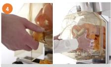
Remove the front cover screws & take off the Front Cover.
