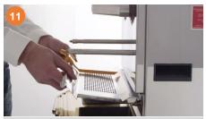
Remove the MTS-System and disassemble the MTS-Pusher. (by pressing the fixation clip)
