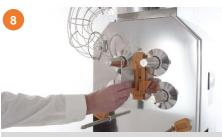
Remove the SCS knife by moving it upward and pulling it off.
