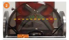
Ensure that the lower pressing elements are in a horizontal position.
