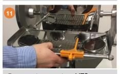
Remove the complete MTS-System (fruit sieve, fruit sieve holder, MTS slider)
