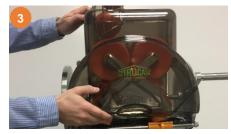
Open the Front Cover fixation screws and take off the Front Cover. CAUTION! Wash only by hand.
