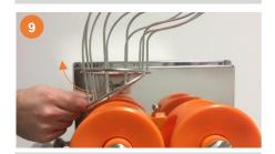
Take off the fruit supply tunnel by opening the fixation lever.
