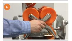
Remove the Cross Holder by loosening and pulling the screw.
