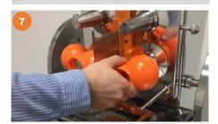
Take off the **lower pressing elements**. During Assembly: Lower pressing elements must be flush with shaft.
