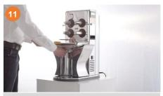
Remove the complete MTS-System (fruit sieve, fruit sieve holder, MTS slider)
