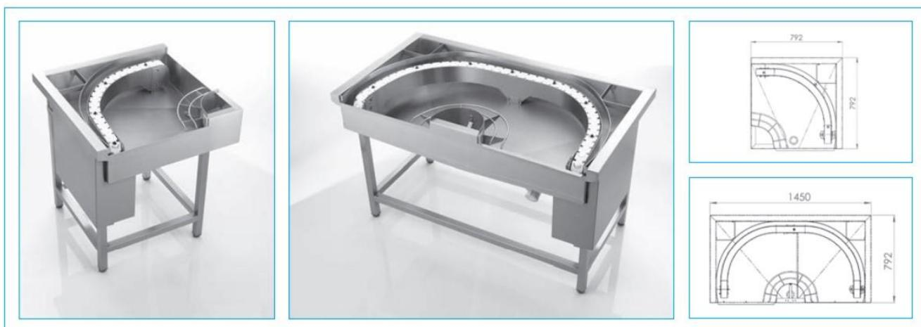
The corner conveyors are available in either 90° or 180° versions and can be used in the draining area of the dishwashing machine. Within the MTR Series they can also be used in the inlet area. The rack conveyor transport is realized by using a link chain.
