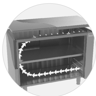
Uniform heat distribution efficient thermal insulation
