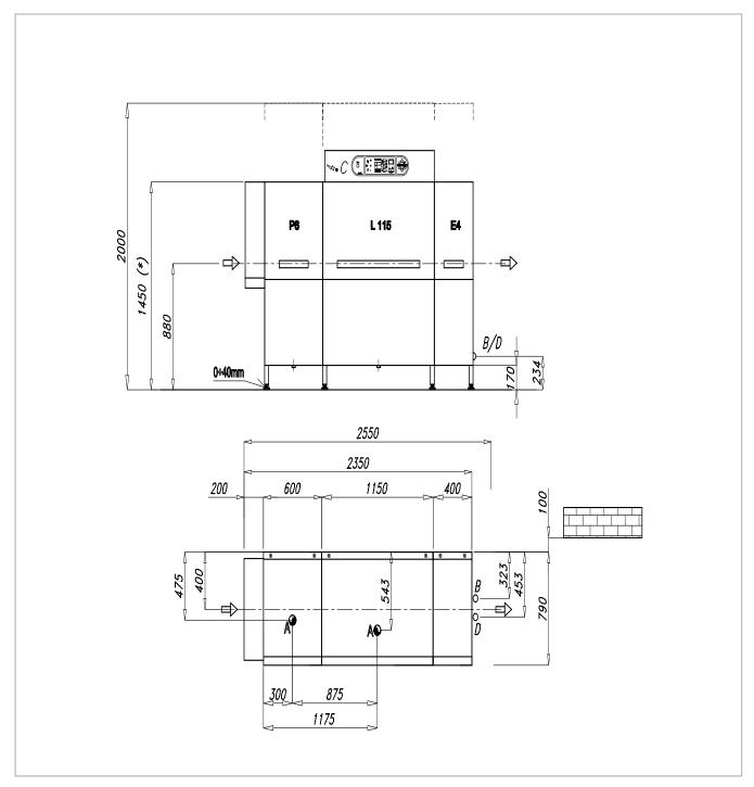
The drawing refers to the standard machine with no optional - Feeding direction: left / right
