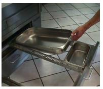
Remove the drawer by placing the drawer to the drawer guide as shown on the picture. Lift the drawer up and remove it. Push the drawer guide back in.
