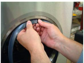
10. Finally check proper placement of the seal in the notch!
