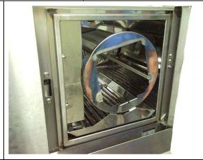
3. Assemble in the new seal. Start with the 4 corners.
