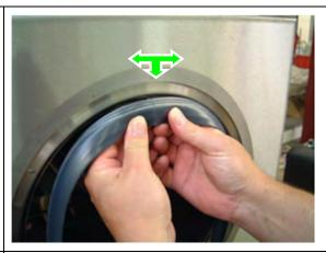
9. Push the seal into the notch. Make sure neither to stretch nor to forge the seal.
