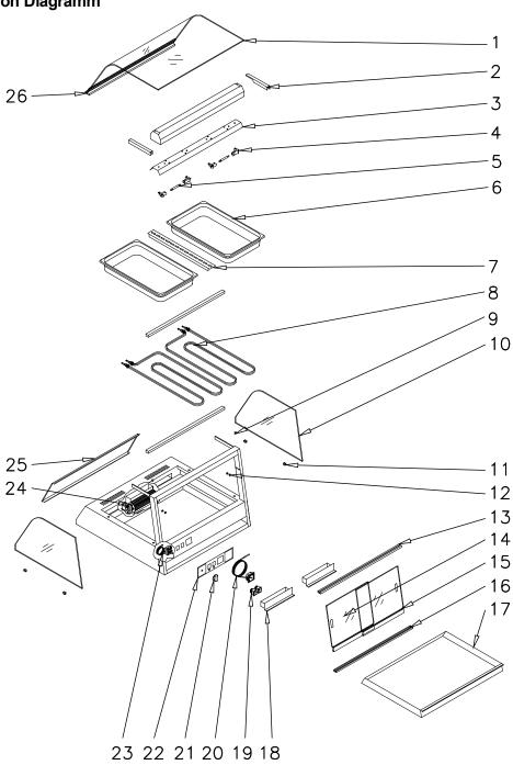
HT and HT DB are almost the same. The only difference is the part 25. It is the front screen on HT and the Dia-Board on HT DB.
