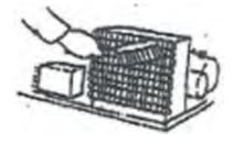
The Deli Cold Cabinet is equipped with a pre-set defrost cycle. The defrost cycle takes place every 4 hours. During the defrost cycle the compressor is switched off while the fans continue to run. The defrost cycle runs until a temperature of 5 °C is reached. The length of the defrost cycle is limited to 30 minutes. If you need to have these settings to be changed, please ask your authorized service technician for guidance.
