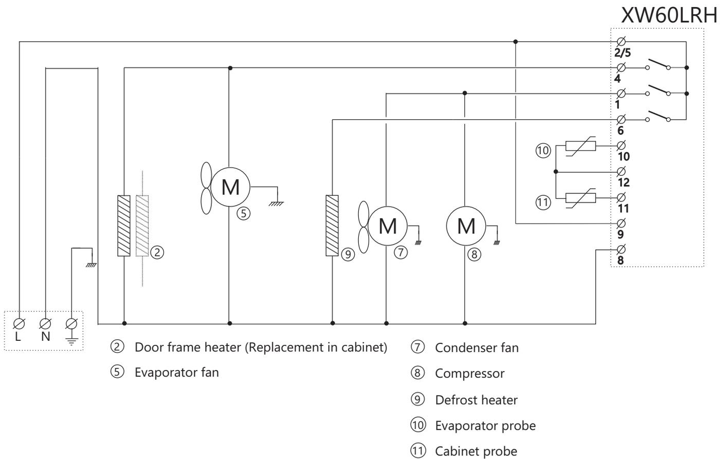
**Digital controller with off cycle defrost and auxiliary relay**
