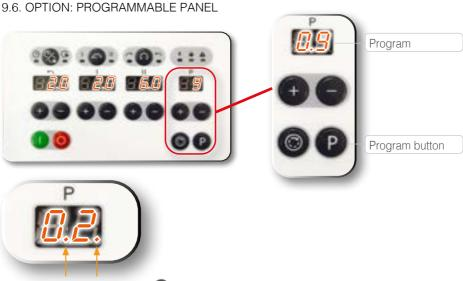
Hold down the program button of for 5 seconds until the two dots start flashing. Use the or button to select the program number you want to set (e.g., 2).
