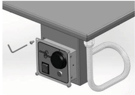
Fig. 7. Positioning control panel into opening
