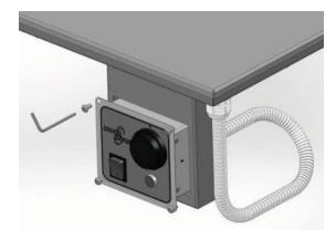
Fig. 7. Positioning control panel into opening
