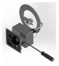
Fig. 3. Replacement of control for heated surface
