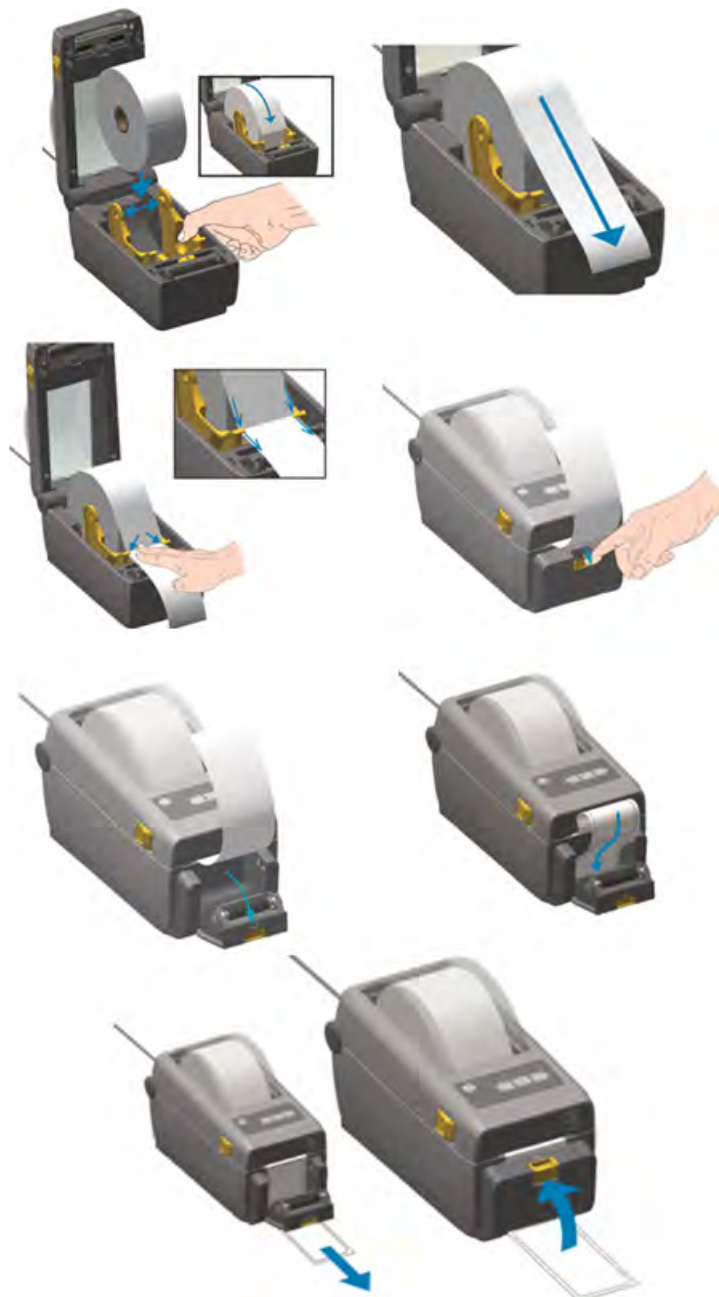
Figure 28: Replacing the Printer Roll
