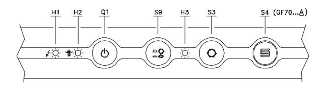
**Q1** Main switch **H1** Pilot lamp "machine ON" **H2** Pilot lamp "machine READY" **H3** Pilot lamp "machine WORKING" **S3** Push button "CYCLE START" **S4** Push button "REGENERATION START" (only mod. GF...A) **S9** Cycle selector S Plug  $\mathbf{S}$ Salt container (only mod. GF...A) Ι Regulating screw for rinse aid injector
