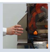
**3.** Remove the side chutes by pressing the fixation clip.
