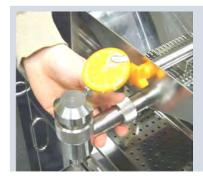
1. Remove tap by unscrewing from machine.
