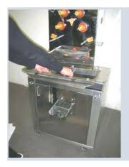
3. The stainless steel cabinet is to be washed with warm water (30 to 50°C) and a cleaning towel. Afterwards dry thoroughly.
