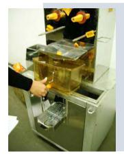
1. Remove the juice tank and wash with warm water (30 bis 50 °C) and cleaning towel.
