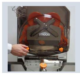
**4.** Remove the fixation screws of the front cover.
