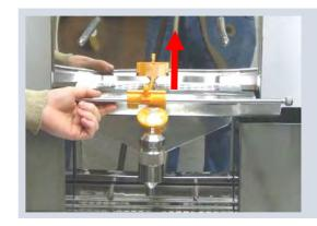
**15.** Remove the MTS-System and disassemble the MTS-Pusher. (Press the fixation clip)
