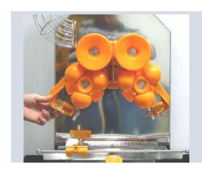
**9.** Remove the peel ejectors (left and right).
