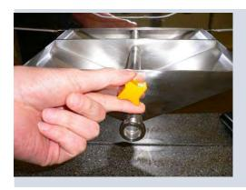
**17.** Unscrew cap-screw to remove fruit sieve. Afterwards wash thoroughly in a sink with warm water or wash in dishwasher.
