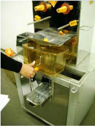
1. Remove the juice tank and wash with warm water (30 bis 50 °C) and cleaning towel.
