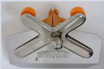
8. Separate the knife guide from the cross holder by pulling out the cross holder screw.
