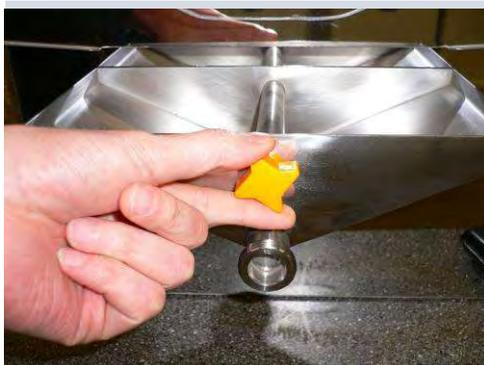
17. Unscrew cap-screw to remove fruit sieve. Afterwards wash thoroughly in a sink with warm water or wash in dishwasher.
