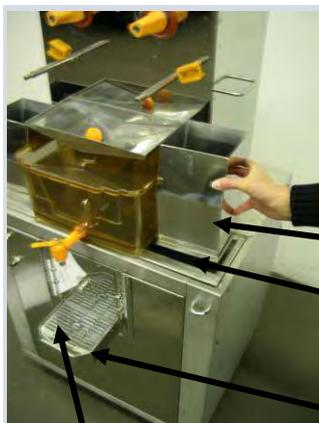
2. Removable parts (such as drip tray, drip plate, peel chute or peel funnel) to be washed in dishwasher or thoroughly washed by hand in the sink.
