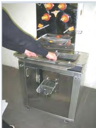
3. The stainless steel cabinet is to be washed with warm water (30 to 50°C) and a cleaning towel. Afterwards dry thoroughly.
