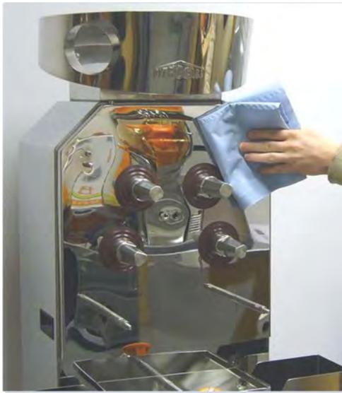
16. Cleaning the housing. Clean the "pressing area" with a cleaning towel and water (30 to 50°C). Clean thoroughly and dry with disposable towels.
