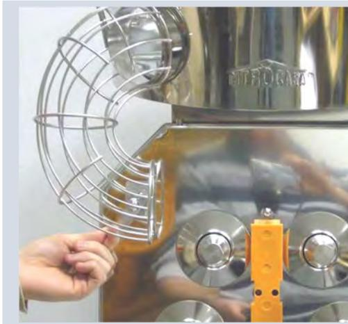
**13.** Open the feeder tube fixation lever and remove the feeder tube.
