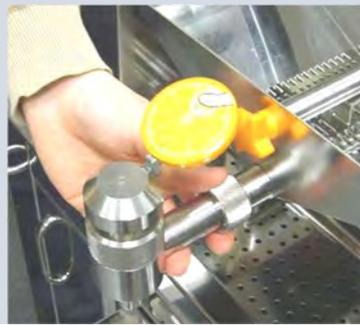
1. Remove tap by unscrewing from machine.
