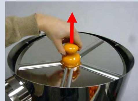
2. Remove the rotary table and place in dishwasher or thoroughly wash by hand in the sink.
