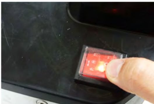
Picture 14: main switch
