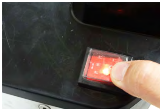
Picture 16: Main switch
