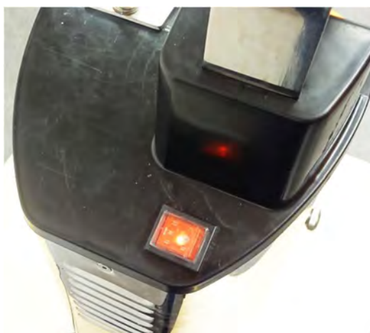
Picture 7: main switch
