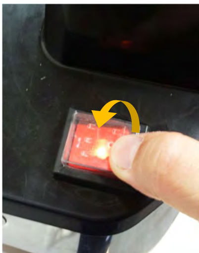
Picture 31: Maschine main switch
