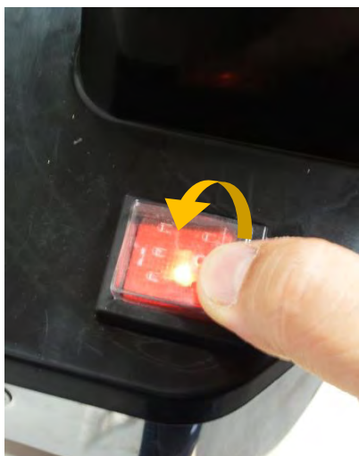
Picture 31: Maschine main switch
