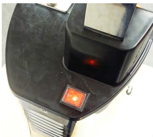
Picture 8: main switch
