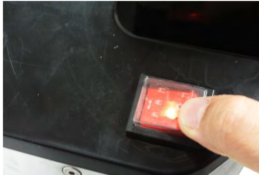
Picture 14: main switch
