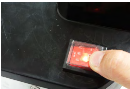
Picture 17: main switch
