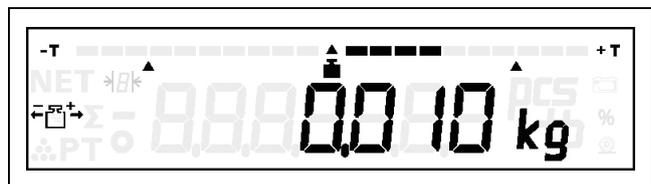
Fig. 16: Weighing against zero
