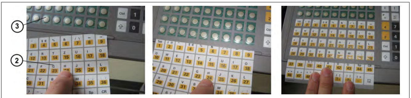
Illustration 13: Insert foil 54 keys
