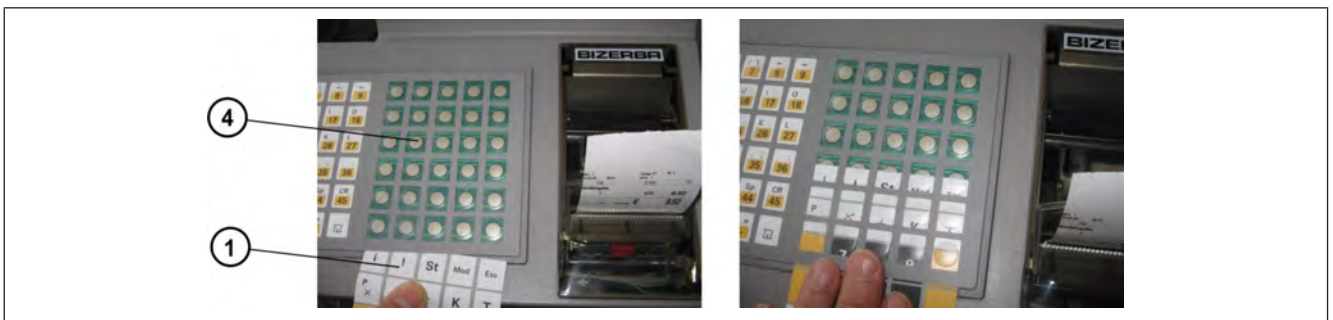
Illustration 14: Insert foil 30 keys
