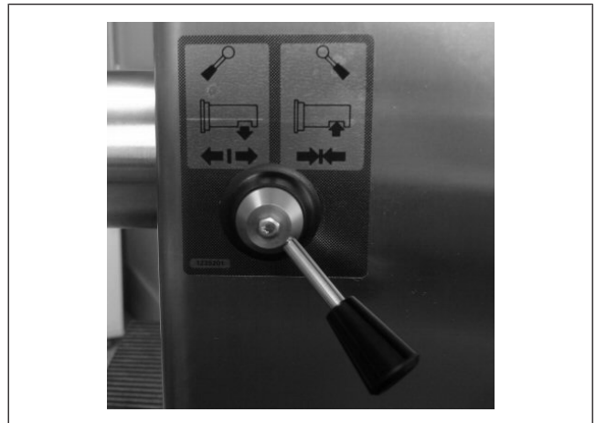
Fig. 9: The worm housing is locked
