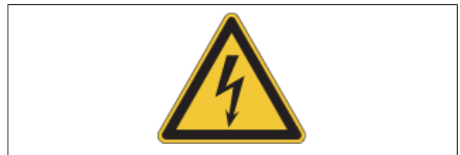
Fig. 4: Warning sign: Flash sign
