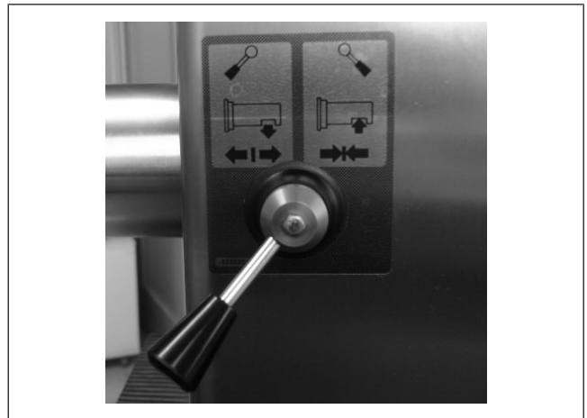
Fig. 8: The worm housing is unlocked
