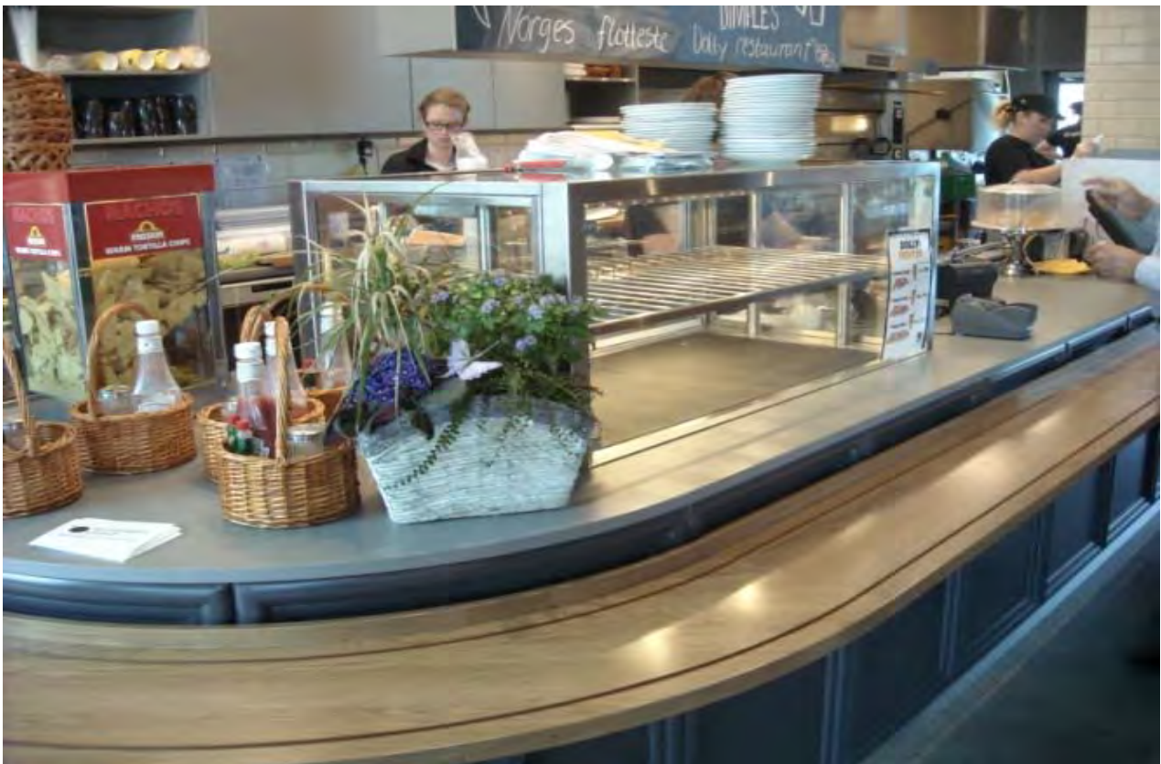
Betjent RBRM monter over varmeplate RBVP
