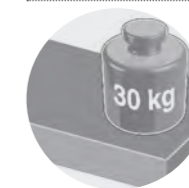
Max loading 30 kg/shelf (uniform layout) Charge max. 30 kg/étagère (disposition uniforme) 30 kg max Tragkraft/Regal
