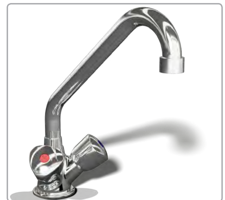
Mixing tap R \frac{3}{4} " (DN 20), emptying 250 mm, outlet height 230 mm (for rectangular cooking kettles 1, 2, 3) Model No. 846101
