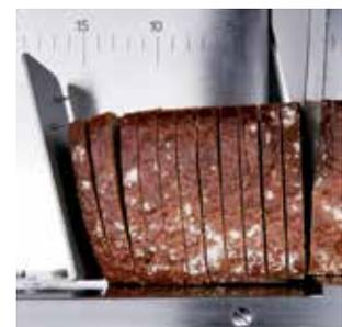
*The slice thickness lies between 3 and 30 mm and can be adjusted via keys during operation. Three save keys enable quick toggling between the three slice thicknesses that can be programmed individually.*
