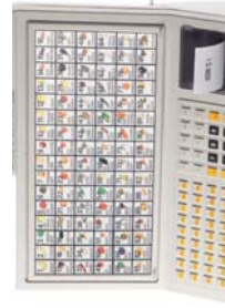
Self-service keyboard with 96 keys and optional operating keyboard (shown with an optional tactile keyboard)
